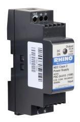
RHINO SELECT PSC series switching power supply, 24 VDC @ 0.63A/15W (adjustable), 120/240 VAC nominal input, 1-phase, enclosed, plastic housing, 35mm DIN rail mount, screw terminals, NEC Class 2.
