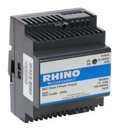
RHINO SELECT PSC series switching power supply, 12 VDC @ 4.5A/54W (adjustable), 120/240 VAC nominal input, 1-phase, enclosed, plastic housing, 35mm DIN rail mount, screw terminals, NEC Class 2.
