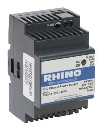
RHINO SELECT PSC series switching power supply, 12 VDC @ 2.5A/30W (adjustable), 120/240 VAC nominal input, 1-phase, enclosed, plastic housing, 35mm DIN rail mount, screw terminals, NEC Class 2.
