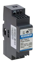
RHINO SELECT PSC series switching power supply, 12 VDC @ 1.25A/15W (adjustable), 120/240 VAC nominal input, 1-phase, enclosed, plastic housing, 35mm DIN rail mount, screw terminals, NEC Class 2.
