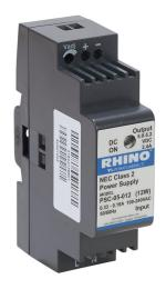
RHINO SELECT PSC series switching power supply, 5 VDC @ 2.4A/12W (adjustable), 120/240 VAC nominal input, 1-phase, enclosed, plastic housing, 35mm DIN rail mount, screw terminals, NEC Class 2.
