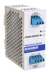
RHINO redundancy module, 2 inputs, 24/48 VDC nominal input, 24-48 VDC output, 20A, alarm contact for operation monitoring, screw terminals, hazardous location rated. Requires (2) matched 24 or 48 VDC power supplies.
