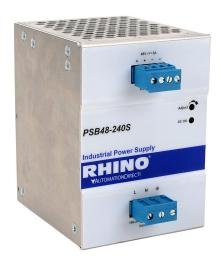
RHINO SELECT PSB series switching power supply, 48 VDC @ 5A/240W (adjustable), 120/240 VAC or 120-375 VDC nominal input, 1-phase, enclosed, aluminum housing, 35mm DIN rail mount, removable screw terminal, hazardous location rated.
