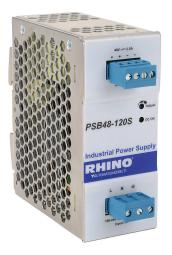
RHINO SELECT PSB series switching power supply, 48 VDC @ 2.5A/120W (adjustable), 120/240 VAC or 120-375 VDC nominal input, 1-phase, enclosed, aluminum housing, 35mm DIN rail mount, removable screw terminal, hazardous location rated.
