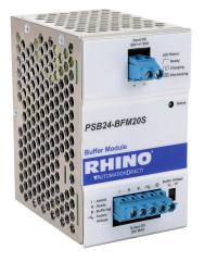
RHINO buffer module, 1 input, 24 VDC nominal input, 23-28 VDC output, 20A, selection switch, alarm contact for operation monitoring, screw terminals, hazardous location rated. Requires PSB24 power supply.
