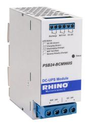
RHINO battery control module, 1 input, 24 VDC nominal input, 23-28 VDC output, 40A, alarm contact for operation monitoring, screw terminals. Requires power supply, 24V battery (usersupplied).
