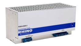
RHINO SELECT PSB series switching power supply, 24 VDC @ 40A/960W (adjustable), 480 VAC nominal input, 3-phase, enclosed, aluminum housing, 35mm DIN rail mount, screw terminals.
