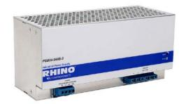
RHINO SELECT PSB series switching power supply, 24 VDC @ 40A/960W (adjustable), 480 VAC nominal input, 3-phase, enclosed, aluminum housing, 35mm DIN rail mount, screw terminals.
