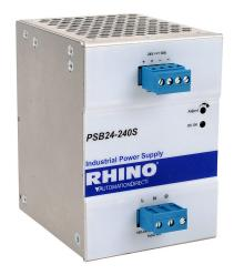
RHINO SELECT PSB series switching power supply, 24 VDC @ 10A/240W (adjustable), 120/240 VAC or 120-375 VDC nominal input, 1-phase, enclosed, aluminum housing, 35mm DIN rail mount, removable screw terminal, hazardous location rated.
