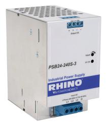
RHINO SELECT PSB series switching power supply, 24 VDC @ 10A/240W (adjustable), 480 VAC nominal input, 3-phase, enclosed, aluminum housing, 35mm DIN rail mount, screw terminals.
