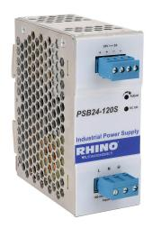
RHINO SELECT PSB series switching power supply, 24 VDC @ 5A/120W (adjustable), 120/240 VAC or 120-375 VDC nominal input, 1-phase, enclosed, aluminum housing, 35mm DIN rail mount, removable screw terminal, hazardous location rated.
