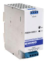
RHINO SELECT PSB series switching power supply, 24 VDC @ 5A/120W (adjustable), 480 VAC nominal input, 3-phase, enclosed, aluminum housing, 35mm DIN rail mount, screw terminals.
