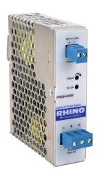
RHINO SELECT PSB series switching power supply, 24 VDC @ 2.5A/60W (adjustable), 120/240 VAC or 120-240 VDC nominal input, 1-phase, enclosed, aluminum housing, 35mm DIN rail mount, removable screw terminal, hazardous location rated.
