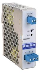
RHINO SELECT PSB series switching power supply, 24 VDC @ 2.5A/60W (adjustable), 120/240 VAC or 120-240 VDC nominal input, 1-phase, enclosed, aluminum housing, 35mm DIN rail mount, removable screw terminal, hazardous location rated.
