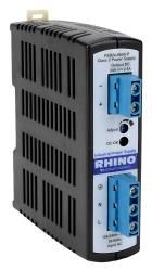
RHINO SELECT PSB series switching power supply, 24 VDC @ 2.5A/60W (adjustable), 120/240 VAC or 120-240 VDC nominal input, 1-phase, enclosed, plastic housing, 35mm DIN rail mount, screw terminals, NEC Class 2, hazardous location rated.
