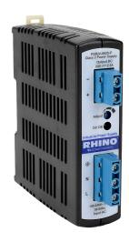
RHINO SELECT PSB series switching power supply, 24 VDC @ 2.5A/60W (adjustable), 120/240 VAC or 120-240 VDC nominal input, 1-phase, enclosed, plastic housing, 35mm DIN rail mount, screw terminals, NEC Class 2, hazardous location rated.
