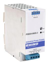
RHINO SELECT PSB series switching power supply, 24 VDC @ 2.5A/60W (adjustable), 480 VAC nominal input, 3-phase, enclosed, aluminum housing, 35mm DIN rail mount, screw terminals.
