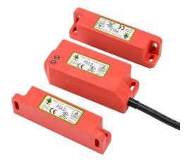
IDEM standalone safety switch set, dual non-contact coded magnetic, manual or automatic restart, (2) N.C. safety output(s), (1) status monitoring output(s), polyester housing, 38mm x 95mm body, pigtail, 32.8ft/10m cable length.
