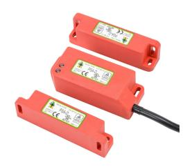
IDEM standalone safety switch set, dual non-contact coded magnetic, manual or automatic restart, (2) N.C. safety output(s), (1) status monitoring output(s), polyester housing, 38mm x 95mm body, pigtail, 16.4ft/5m cable length.
