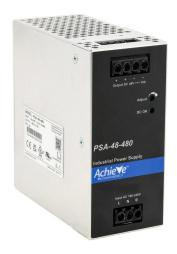
AchieVe PSA series switching power supply, 48 VDC @ 10A/480W, 120/240 VAC nominal input, 1-phase, enclosed, aluminum housing, 35mm DIN rail mount, screw terminals.
