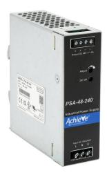
AchieVe PSA series switching power supply, 48 VDC @ 5A/240W, 120/240 VAC nominal input, 1-phase, enclosed, aluminum housing, 35mm DIN rail mount, screw terminals.
