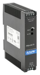
AchieVe PSA series switching power supply, 24 VDC @ 3.125A/75W, 120/240 VAC nominal input, 1-phase, enclosed, plastic housing, 35mm DIN rail mount, screw terminals.
