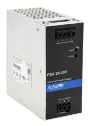
AchieVe PSA series switching power supply, 24 VDC @ 20A/480W, 120/240 VAC nominal input, 1-phase, enclosed, aluminum housing, 35mm DIN rail mount, screw terminals.
