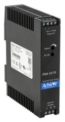
AchieVe PSA series switching power supply, 12 VDC @ 6.2A/75W, 120/240 VAC nominal input, 1-phase, enclosed, plastic housing, 35mm DIN rail mount, screw terminals.
