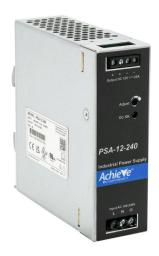
AchieVe PSA series switching power supply, 12 VDC @ 20A/240W, 120/240 VAC nominal input, 1-phase, enclosed, aluminum housing, 35mm DIN rail mount, screw terminals.
