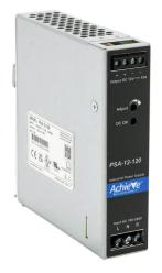
AchieVe PSA series switching power supply, 12 VDC @ 10A/120W, 120/240 VAC nominal input, 1-phase, enclosed, aluminum housing, 35mm DIN rail mount, screw terminals.
