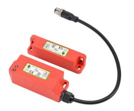
IDEM standalone safety switch set, non-contact coded magnetic, manual restart, (2) N.C. safety output(s), polyester housing, 38mm x 95mm body, 8-pin M12 quick-disconnect, 9.8in/250mm cable length.
