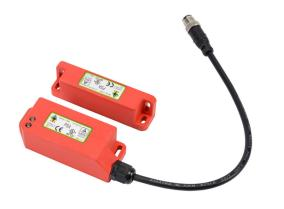
IDEM standalone safety switch set, non-contact coded magnetic, automatic restart, (2) N.C. safety output(s), polyester housing, 38mm x 95mm body, 8-pin M12 quick-disconnect, 9.8in/250mm cable length.
