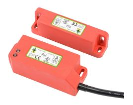
IDEM standalone safety switch set, non-contact coded magnetic, manual or automatic restart, (2) N.C. safety output(s), (1) status monitoring output(s), polyester housing, 38mm x 95mm body, pigtail, 32.8ft/10m cable length.
