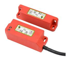
IDEM standalone safety switch set, non-contact coded magnetic, manual or automatic restart, (2) N.C. safety output(s), (1) status monitoring output(s), polyester housing, 38mm x 95mm body, pigtail, 16.4ft/5m cable length.
