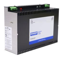
RHINO SELECT PS series switching power supply, 24 VDC @ 24A/576W (adjustable), 120/240 VAC nominal input, 1-phase, enclosed, metal housing, 35mm DIN rail mount, removable screw terminal, hazardous location rated.
