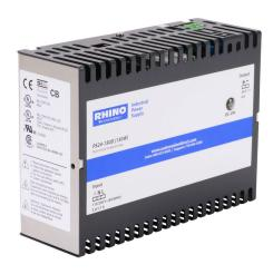
RHINO SELECT PS series switching power supply, 24 VDC @ 6A/144W (adjustable), 120/240 VAC nominal input, 1-phase, enclosed, metal housing, 35mm DIN rail mount, removable screw terminal, hazardous location rated.
