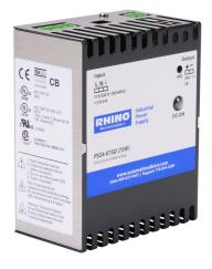
RHINO SELECT PS series switching power supply, 24 VDC @ 3A/72W (adjustable), 120/240 VAC nominal input, 1-phase, enclosed, metal housing, 35mm DIN rail mount, removable screw terminal, hazardous location rated.
