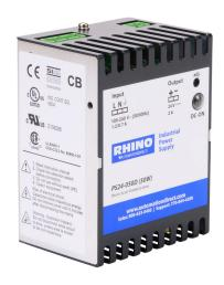
RHINO SELECT PS series switching power supply, 24 VDC @ 2A/48W (adjustable), 120/240 VAC nominal input, 1-phase, enclosed, metal housing, 35mm DIN rail mount, removable screw terminal.
