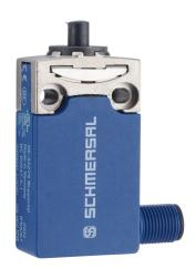
Schmersal compact limit switch, plastic plunger, 45-degree adjustable head, (1) N.O./(1) N.C. contact(s), snap action, 20-22mm hole spacing, die-cast zinc with plastic base, (1) 4-pin M12 quick-disconnect, right exit.
