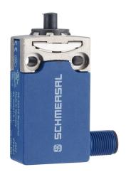
Schmersal compact limit switch, plastic plunger, 45-degree adjustable head, (1) N.O./(1) N.C. contact(s), snap action, 31mm wide body, 20-22mm hole spacing, die-cast zinc with plastic base, 4-pin M12 quick-disconnect, right exit.
