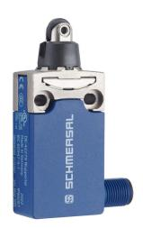
Schmersal compact limit switch, plunger with plastic roller, 45-degree adjustable head, (1) N.O./(1) N.C. contact(s), snap action, 31mm wide body, 20-22mm hole spacing, die-cast zinc with plastic base, 4-pin M12 quick-disconnect, right exit.
