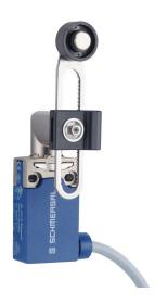
Schmersal compact limit switch, side rotary adjustable lever with plastic roller, 45-degree adjustable head, (1) N.O./(1) N.C. contact(s), snap action, 31mm wide body, 20-22mm hole spacing, die-cast zinc with plastic base, pigtail, 6.5ft/2m cable length, right exit.
