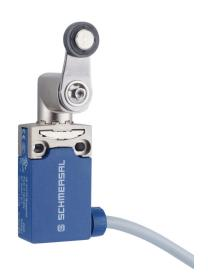
Schmersal compact limit switch, side rotary lever with plastic roller, 45-degree adjustable head, (1) N.O./(1) N.C. contact(s), snap action, 31mm wide body, 20-22mm hole spacing, die-cast zinc with plastic base, pigtail, 6.5ft/2m cable length, right exit.
