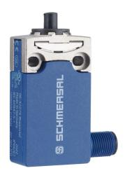
Schmersal compact limit switch, plastic plunger, 45-degree adjustable head, (1) N.O./(1) N.C. contact(s), slow action break before make, 31mm wide body, 20-22mm hole spacing, die-cast zinc with plastic base, 4-pin M12 quick-disconnect, right exit.
