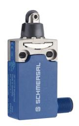
Schmersal compact limit switch, plunger with plastic roller, 45-degree adjustable head, (1) N.O./(1) N.C. contact(s), slow action break before make, 31mm wide body, 20-22mm hole spacing, die-cast zinc with plastic base, 4-pin M12 quick-disconnect, right exit.
