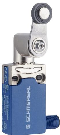
Schmersal compact limit switch, side rotary lever with plastic roller, 45-degree adjustable head, (1) N.O./ (1) N.C. contact(s), slow action break before make, 20-22mm hole spacing, die-cast zinc with plastic base, (1) 4-pin M12 quick-disconnect, right exit.
