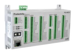
ProductivityMotion 4-axis motion controller, 1 MHz maximum switching frequency, 24 high-speed input point(s), sinking, 4-channel, differential encoder input(s), 12 high-speed output point(s), sinking/sourcing, 4-channel, differential output(s).
