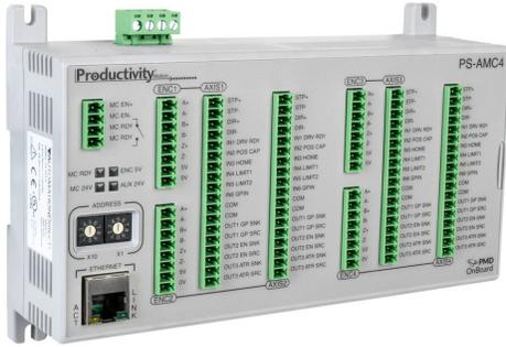
ProductivityMotion 4-axis motion controller, 1 MHz maximum switching frequency, 24 high-speed input point(s), sinking, 4-channel, differential encoder input(s), 12 high-speed output point(s), sinking/sourcing, 4-channel, differential output(s).
