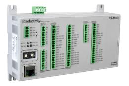
ProductivityMotion 3-axis motion controller, 1 MHz maximum switching frequency, 18 high-speed input point(s), sinking, 3-channel, differential encoder input(s), 9 high-speed output point(s), sinking/sourcing, 3-channel, differential output(s).
