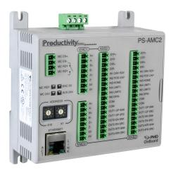
ProductivityMotion 2-axis motion controller, 1 MHz maximum switching frequency, 12 high-speed input point(s), sinking, 2-channel, differential encoder input(s), 6 high-speed output point(s), sinking/sourcing, 2-channel, differential output(s).
