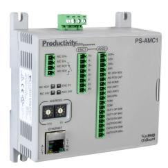
ProductivityMotion 1-axis motion controller, 1 MHz maximum switching frequency, 6 high-speed input point(s), sinking, 1-channel, differential encoder input(s), 3 high-speed output point(s), sinking/sourcing, 1-channel, differential output(s).
