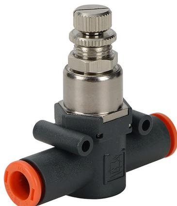
NITRA pneumatic push-to-connect fitting, inline pressure regulator, technopolymer body, (1) 5/16in (8mm) push-to-connect inlet(s), (1) 5/16in (8mm) push-to-connect outlet(s), 15-120 psi adjustable range.
