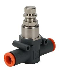
NITRA pneumatic push-to-connect fitting, inline pressure regulator, technopolymer body, 5/16in (8mm) tube inlet(s), 5/16in (8mm) tube outlet(s), 15-120 psi adjustable range.
