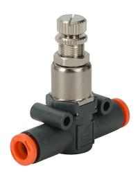
NITRA pneumatic push-to-connect fitting, inline pressure regulator, technopolymer body, (1) 1/4in push-to-connect inlet(s), (1) 1/4in push-to-connect outlet(s), 15-120 psi adjustable range.
