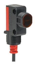
Leuze photoelectric sensor, rectangular, polarized retroreflective, visible red, 0.02-4.5m sensing distance, complementary light-on/dark-on, PNP, 4-wire, pigtail.
