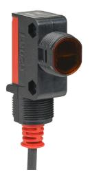
Leuze photoelectric sensor, rectangular, polarized retroreflective, visible red, 0.02-4.5m sensing distance, complementary light-on/ dark-on, PNP, 4-wire, 4-pin M12 quick-disconnect.
