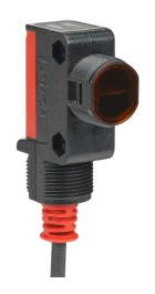
Leuze photoelectric sensor, rectangular, polarized retroreflective, visible red light emission, 0.02-4.5m sensing distance, complementary light-on/dark-on, PNP, 4-wire, 4-pin M12 quick-disconnect.
